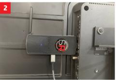
Plug the Server into your TV HDMI port. It can also be mounted on back of TV with velcro. Turn TV on with volume up.
